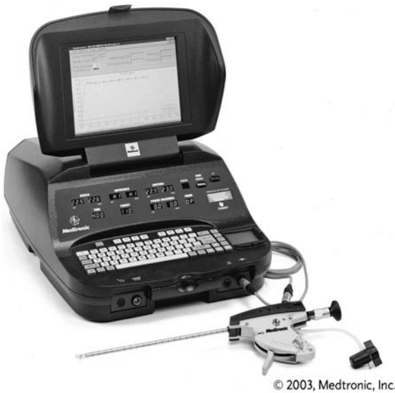
Figure 27 Precision™ Plus System (computer and hand piece).
